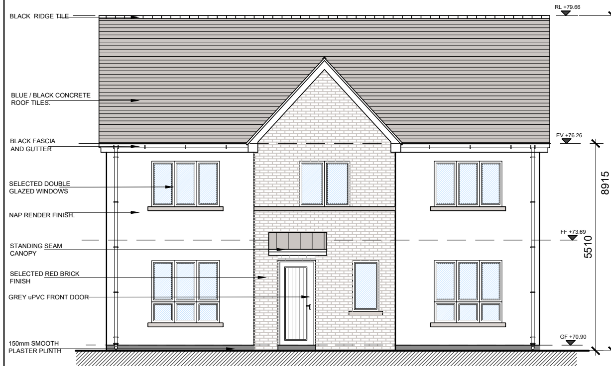
FRONT ELEVATION SCALE 1:100
